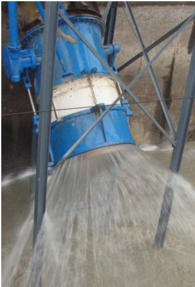
Without hood, flow spray out evenly to a large area.
