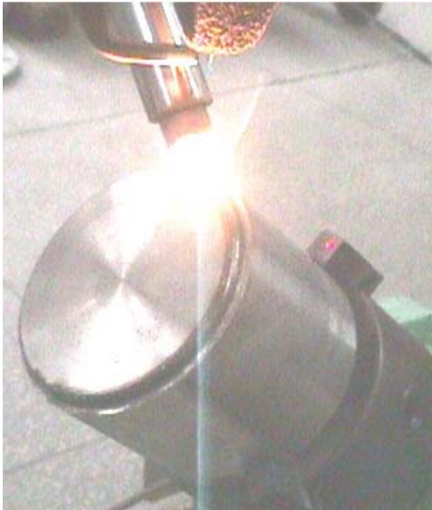
Using laser cladding technology to apply the Nickel layer.
